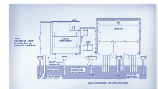
Side view of Brilliant Rack Pad Support featuring patented helical piles. New concrete pads or steel skids can easily be installed to a specified height above grade to brackets attached to the top of helical piles.
